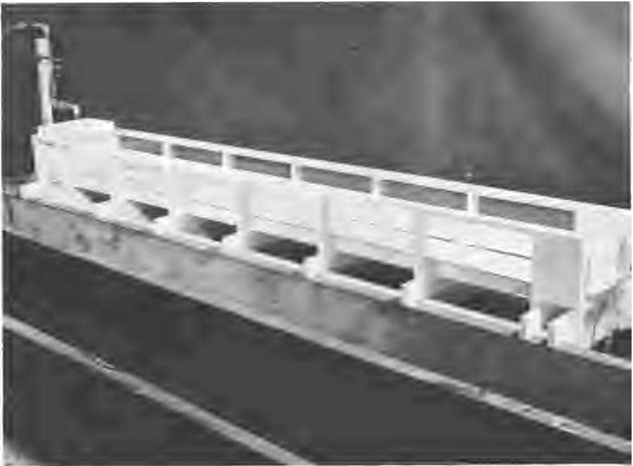
Figure 3.—Model of the raceway pond. The two plastic plates in the foreground were added to facilitate capture of the effluent.
