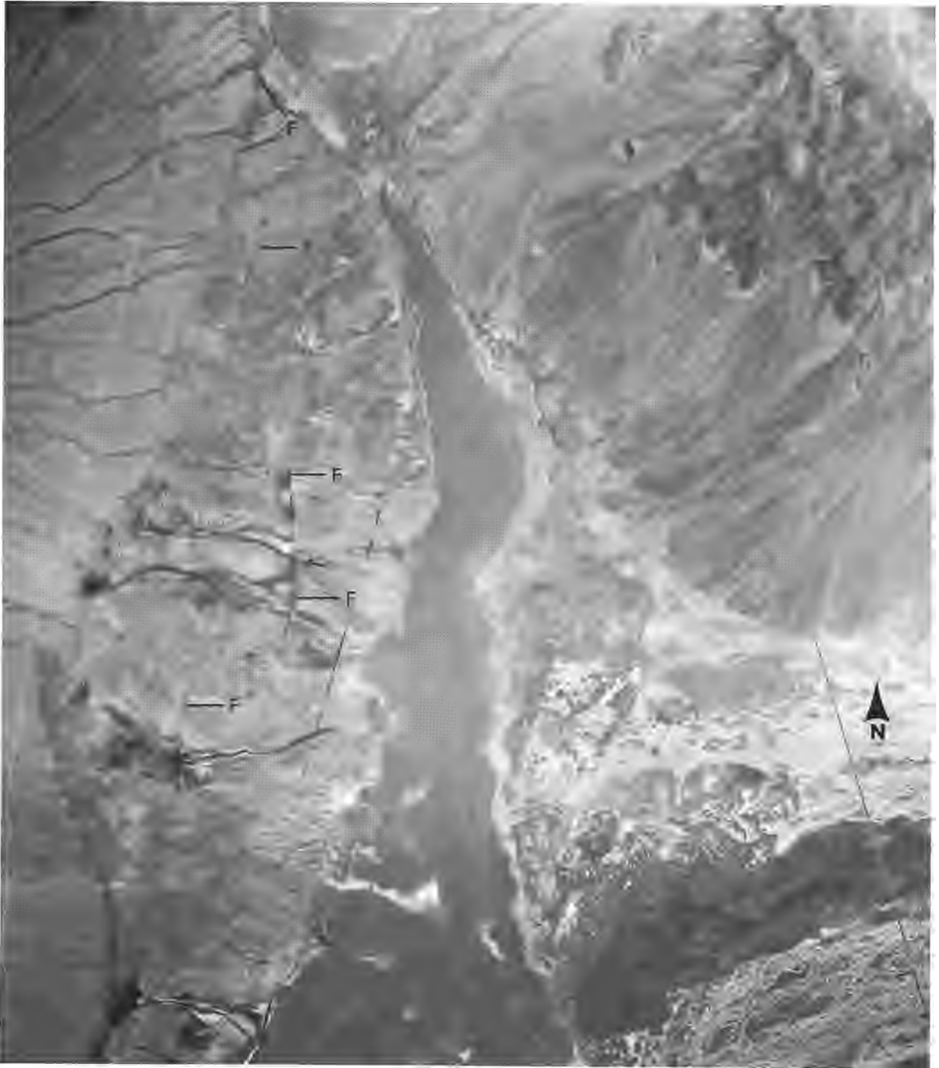
FIGURE 13. View of the north end of Steptoe Valley south of Currie where a series of faults (F) localize groundwater discharge and create lineations. This area is the lowest part of Steptoe Valley and absence of Lahontan age shoreline features on the northwest flank of the valley helps confirm the origin of lineations in the valley which might be confused with shoreline features.
