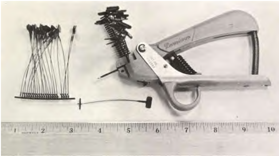
New tagging device is compact and faster than previous jaw or fin clipping methods.
