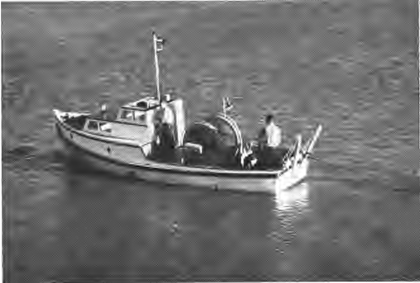
FIGURE 2. The Striper , 28-foot Fraser River type gill-netter used for striped bass tagging work
