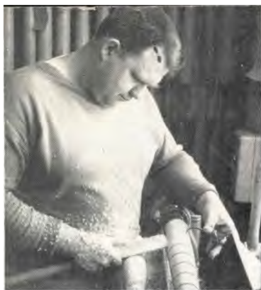
Billet is shaped on lathe, calipered to proper dimension
