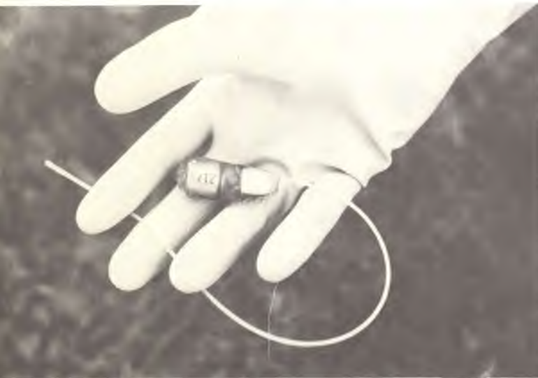
Figure 16. Making a tunnel under the skin for the whip antenna. The antenna is connected to the tunneling tool by a thread and follows the tool into the tunnel.
