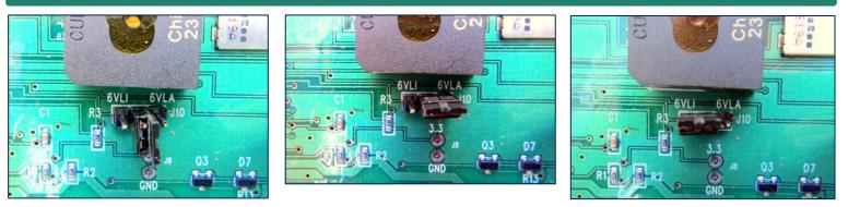
Varying jumper placement on logger depending on battery type. Jumpers located next to buzzer on gray box and next to communication cable port on mini logger.
