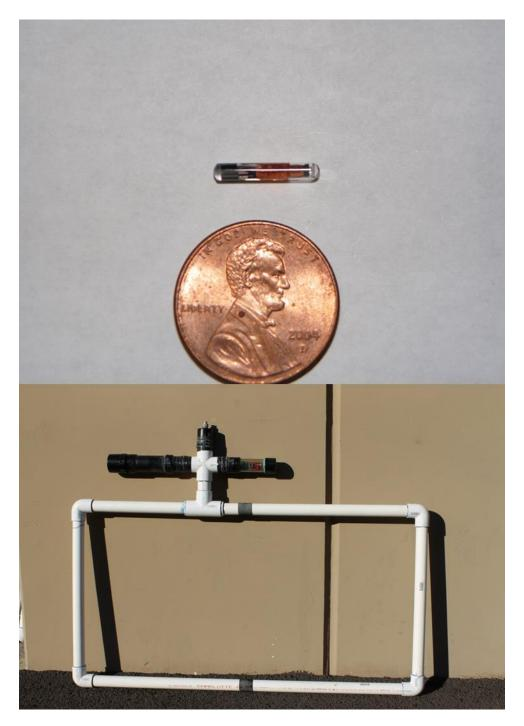
Figure 7. Remote PIT scanning equipment used during the 2013 June sucker study. Top photo is an example of the 134 kHz PIT tag that was implanted in the study fish. Bottom photo is the submersible PIT scanning unit deployed throughout the lake.
