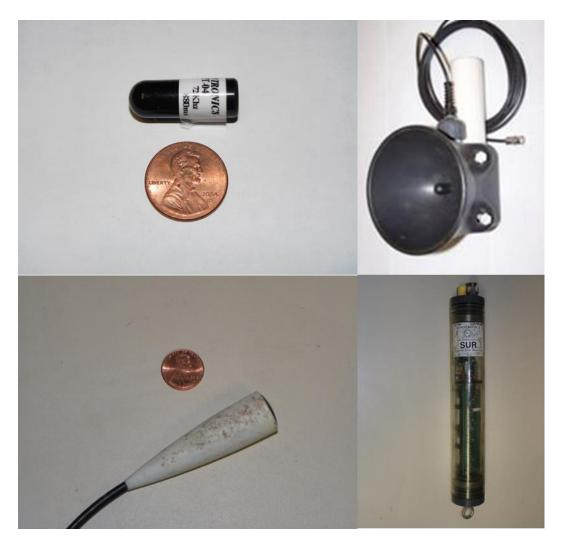
Figure 2. Telemetry equipment used for the June sucker study. Upper left photo is the Sonotronics Inc. (Tucson, Arizona) model PT-4 acoustic tag. Upper right photo is the directional hydrophone (Sonotronics model DH-4). Lower left photo is the omni-directional towable hydrophone (Sonotronics model TH-2). Lower right photo is the Sonotronics Inc. (Tucson, Arizona) Submersible Ultrasonic Receiver.
