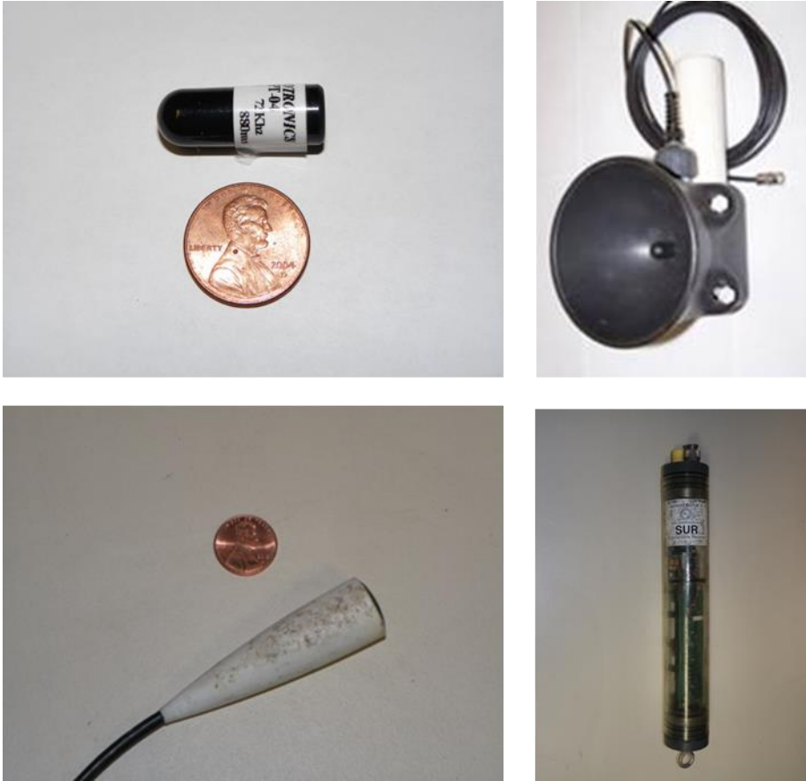
Figure 2. Telemetry equipment used for the June sucker study. Upper left: Sonotronics Inc. (Tucson, Arizona) model PT-4 acoustic tag; Upper right: directional hydrophone (Sonotronics model DH-4); Lower left: omni-directional towable hydrophone (Sonotronics model TH-2); Lower right: Sonotronics Inc. (Tucson, Arizona) Submersible Ultrasonic Receiver (SUR).
